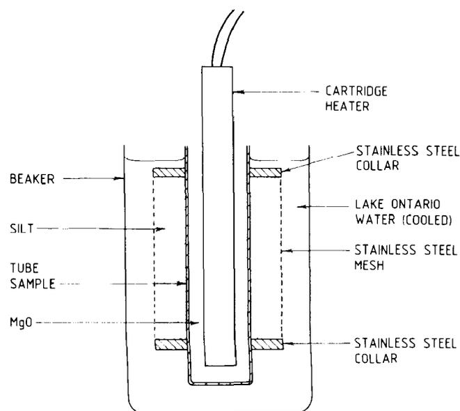
**Figure 1:** Schematic of test apparatus used for corrosion tests with heat transfer and silt crevices. The stainless steel used for collars and mesh was type 304.
