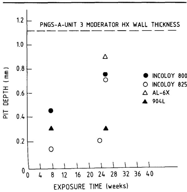
**Figure 2:** Average maximum pit depths for moderator heat exchanger tube materials subjected to laboratory testing in Lake Ontario water.
