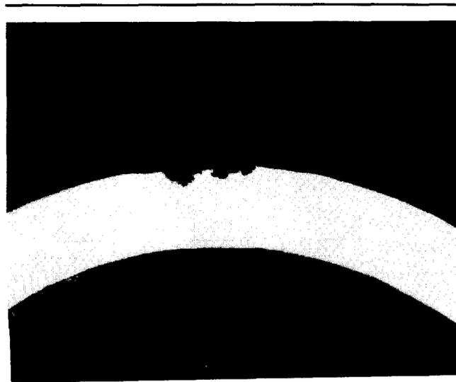
**Figure 3:** Typical deep pit in Incoloy 800 after two months' exposure to Lake Ontario water (with a crevice).
